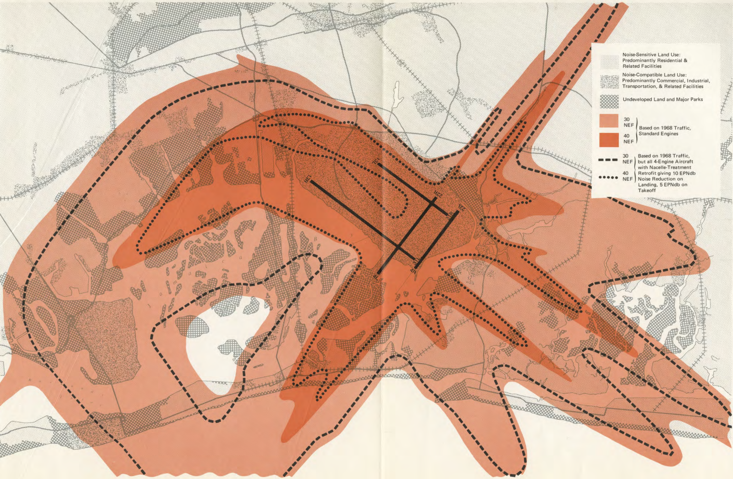
FIGURE 4-6 Comparison of noise-exposure contours under present conditions and with nacelle-treatment retrofit. Scale: 1" = 1 Mile
